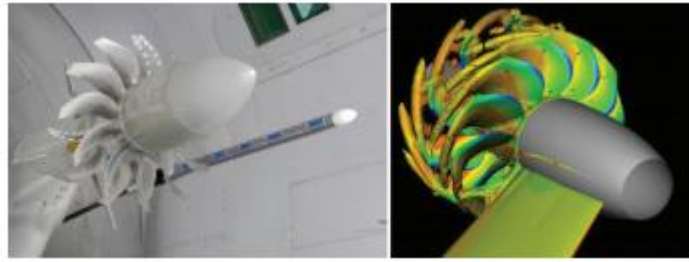
Figure 4.101: Open Rotor mounted on Hera vehicle (Sneema) and under test at the S1 Onera wind tunnel and the simulation of interactions between the two propellers (Onera)
