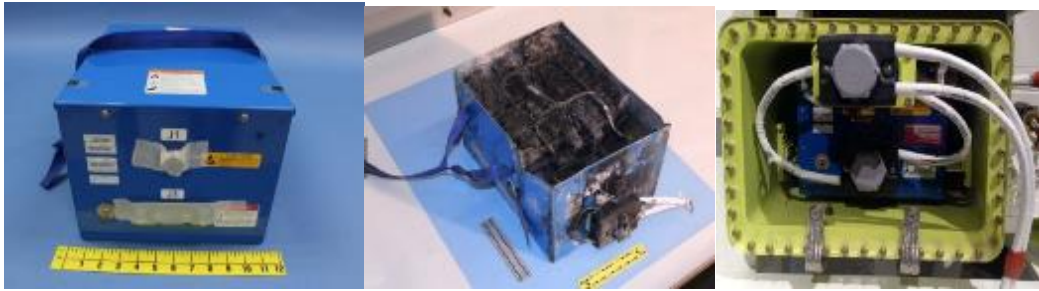
Figure 4.108: Boeing-787 relaunched the Li-ion battery system with the new design, adding an extra weight of 68kg to the weight of the airplane
