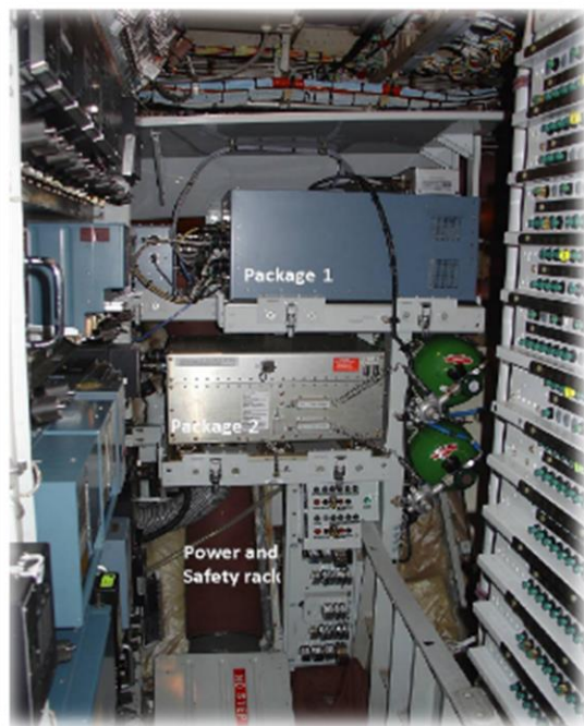
Figure 4.137: Instrumentation installed in aircraft for environmental purpose
