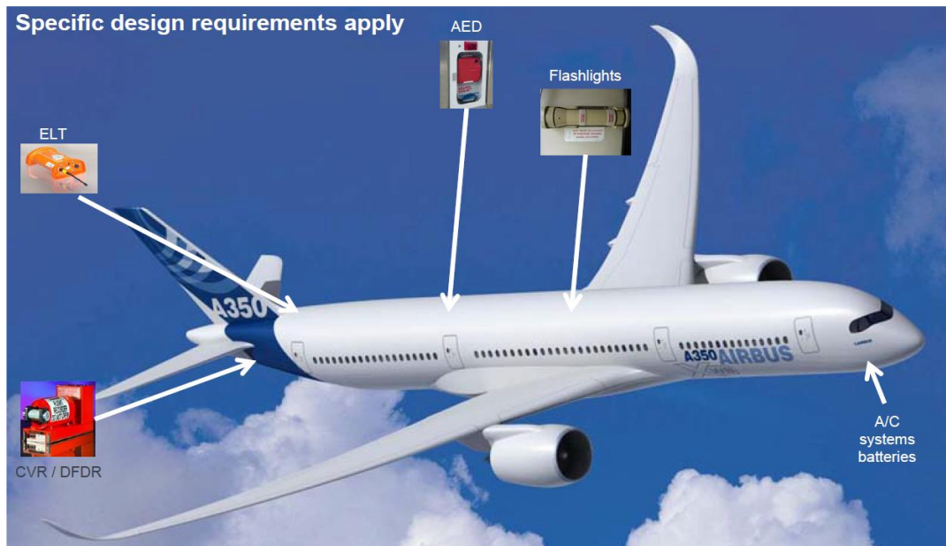
Figure 4.109: Use of batteries in a typical aircraft
