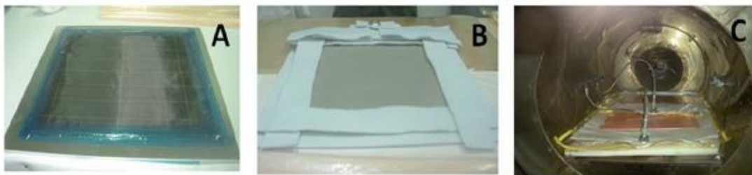
Figure 8.36 - Steps for the preparation of laminates adopted in IASS project "Source - L. Guadagno et al. RSC Adv., 2015, 5, 6033, DOI: 10.1039/c4ra12156b
