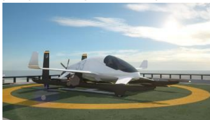
Figure 2.59. Aurora's VTOL aircraft use eight lifting propellers for vertical take-off, and a cruise propeller and wing to transition to high-speed forward cruise.
