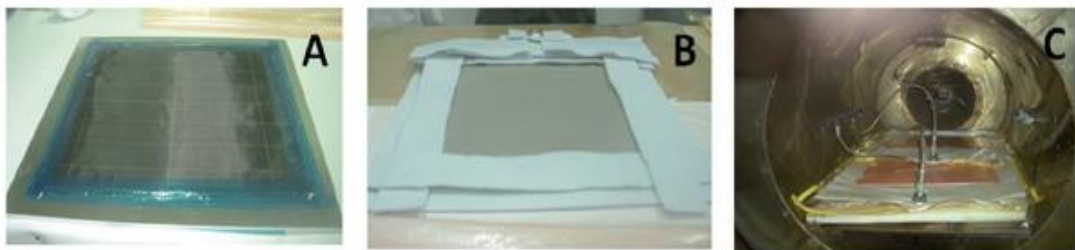
Figure 8.57 - Steps for the preparation of laminates adopted in the IASS project "Source - L. Guadagno et al. RSC Adv., 2015, 5, 6033, DOI: 10.1039/c4ra12156b
