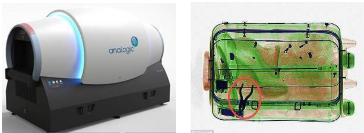
Figure 5.74 – Computer tomography scanning creates 3-Dimension Image
