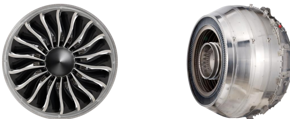
Figure 35. Carbon fibre composite fan blades and advanced low-pressure turbine (LPT)
