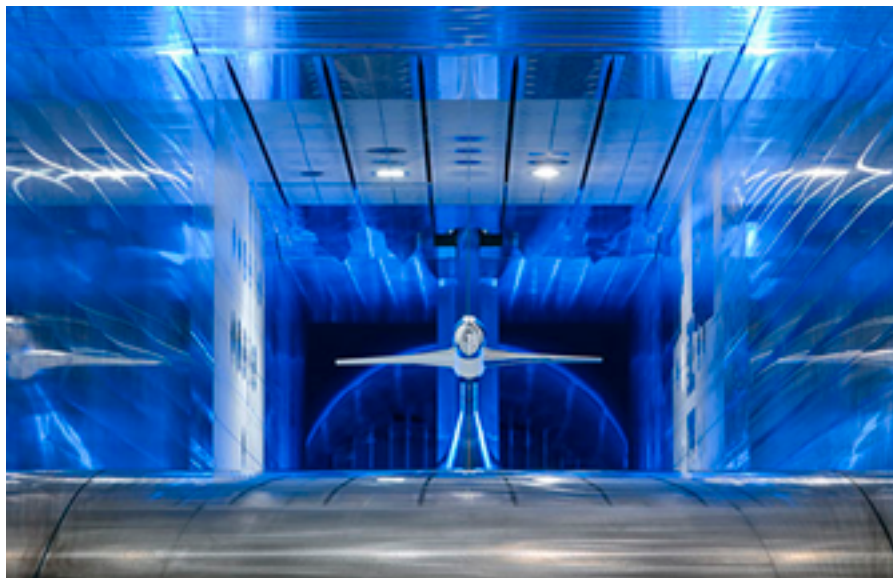
Figure 17 - Downstream view into Test Section of the European transonic wind tunnel (ETW).
