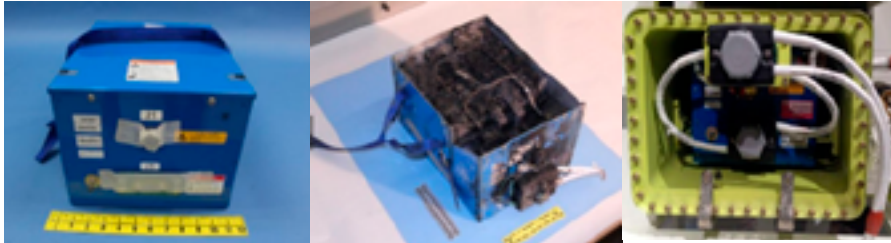
Figure 8 - Boeing-787 relaunched the Li-ion battery system with the new design, adding an extra weight of 68kg to the weight of the airplane.
