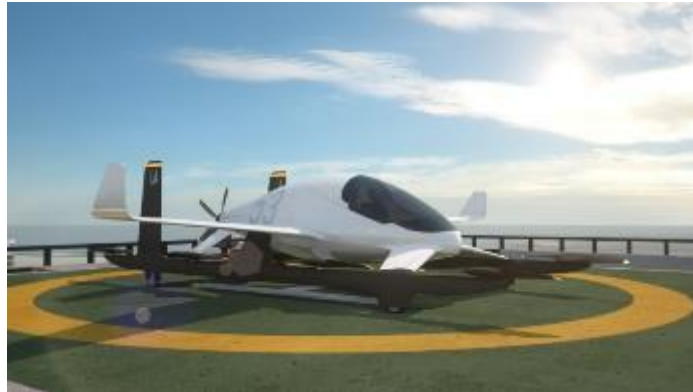
Figure 2.52 - Aurora's VTOL aircraft use eight lifting propellers for vertical take-off, and a cruise propeller and wing to transition to high-speed forward cruise.
