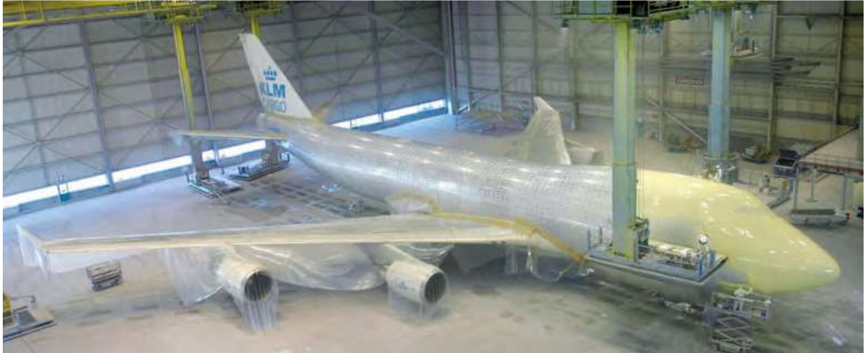
Figure 34. Painting process at KLM
