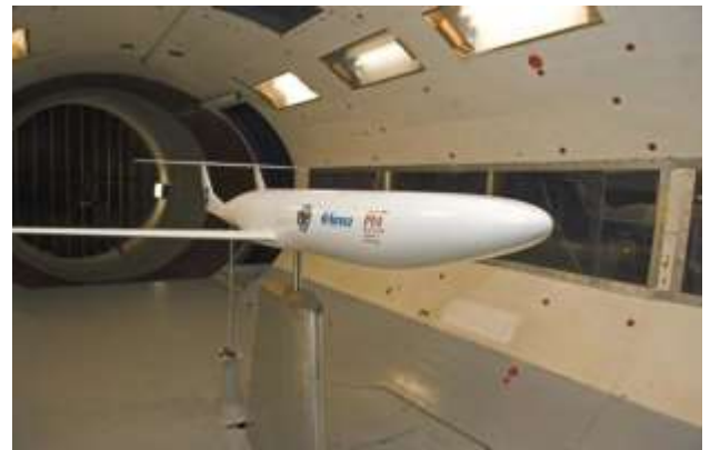
Figure 70. Experimental studies of BLI characteristics
