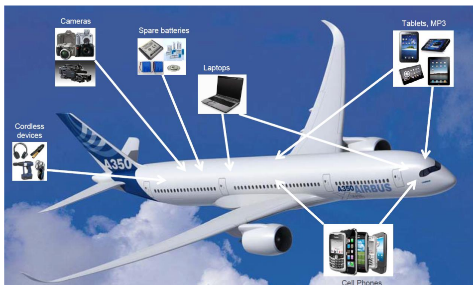
Figure 4.36 – Batteries in the cabin of an airliner
