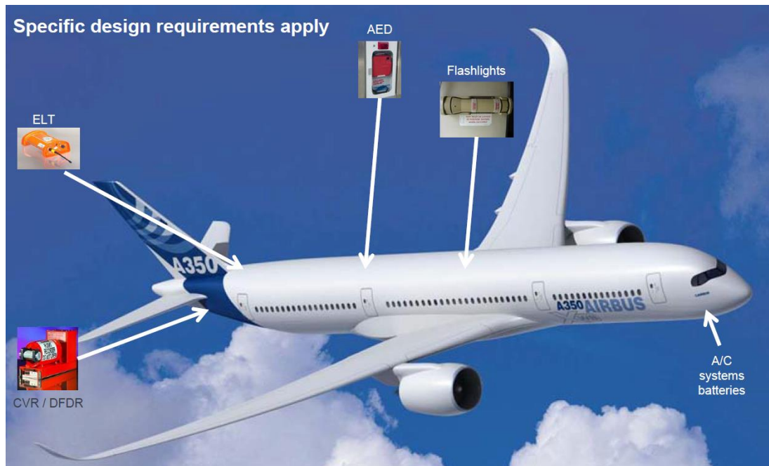
Figure 4.35 – Use of batteries in a typical aircraft.
