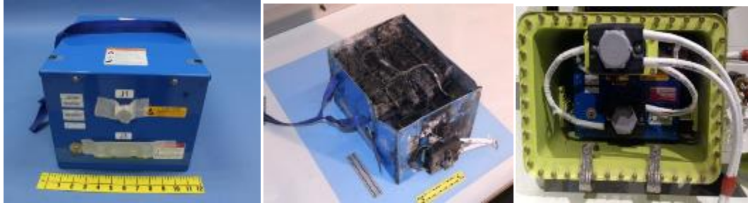
Figure 4.34 - Boeing-787 relaunched the Li-ion battery system with the new design, adding an extra weight of 68kg to the weight of the airplane.
