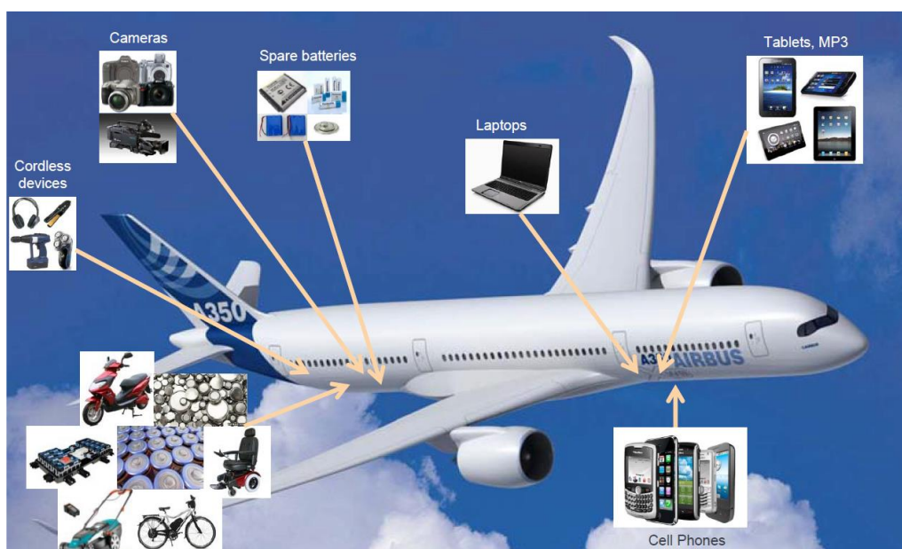
Figure 4.37 – Cargo with batteries that can cause safety risks
